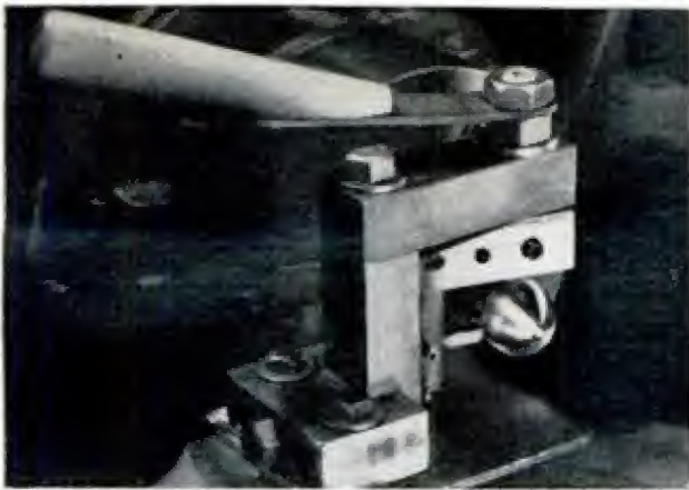
TWO 1/4-IN. BOLTS hold the attachment in position over the toolpost slot of the lathe carriage
